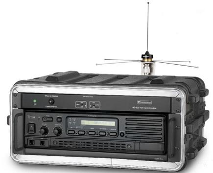
Production Intercom's Wireless Intercom Solution is a base unit combining the HD903 adapter and 50 watt FR4000 for integrating wireless UHF handhelds and a wired intercom system.
